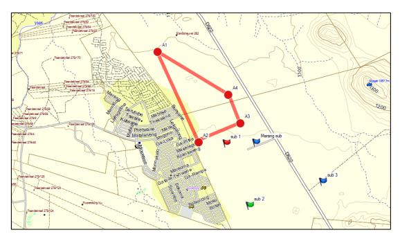
Figure 8: Site for Alternative 1 substation (red flag) and the corridor for power line (red box).
